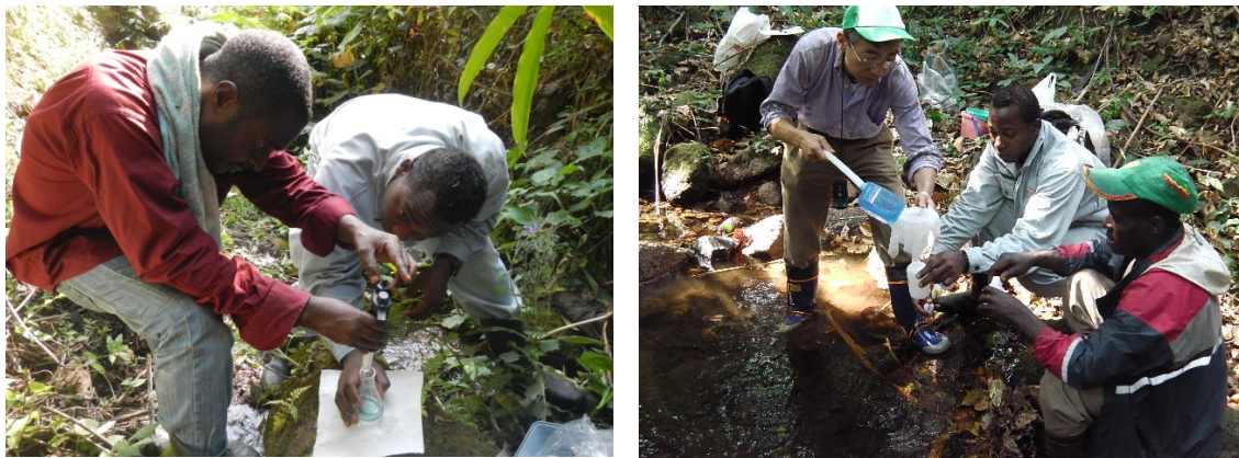
Fig. 2 In-situ measurements of alkalinity and sampling
