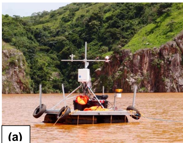
Figure 6. (a) Climate station (2.5m×2.5m) and (b) work raft (3.2m×3.2m) at Lake Nyos, June 2012.
