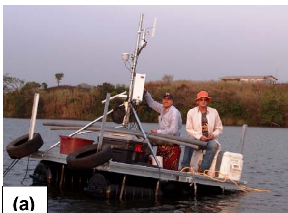
Figure 7. (a) Climate station (2.5m×2.5m) and (b) work raft (2.5m×2.5m) at Lake Monoun, January 2013.
